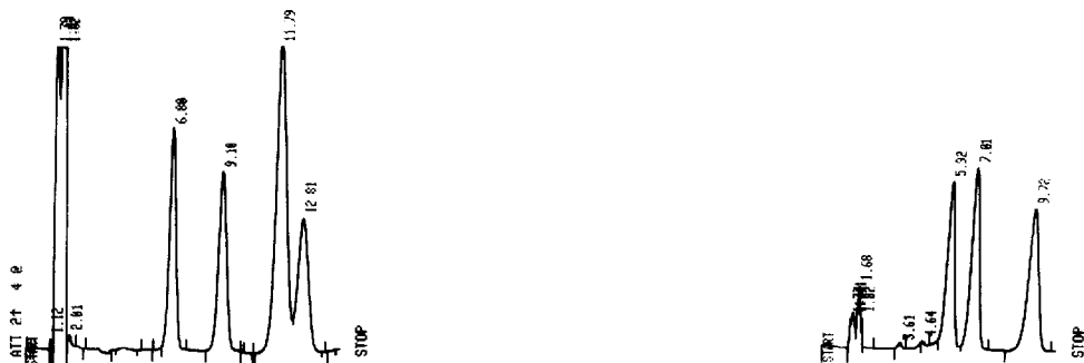
Fig. 1. HPLC separation of aromatic monomethoxy acids. Column: Nucleosil C_{18} , 5 \mu m , 200 \times 4 mm. Mobile phase: acetonitrile-0.1 M phosphate buffer (pH 2) (20:80). Flow-rate: 1.5 ml/min. Detection: UV at 240 nm. Elution order: 2-methoxybenzoic, benzoic, 4-methoxybenzoic and 3-methoxybenzoic acid at 6.8, 9.1, 11.79 and 12.81 min respectively.
